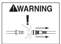
Always disconnect air from stapler whenever servicing! During maintenance, a stapler connected to air may fire accidentally, causing serious personal injury!
